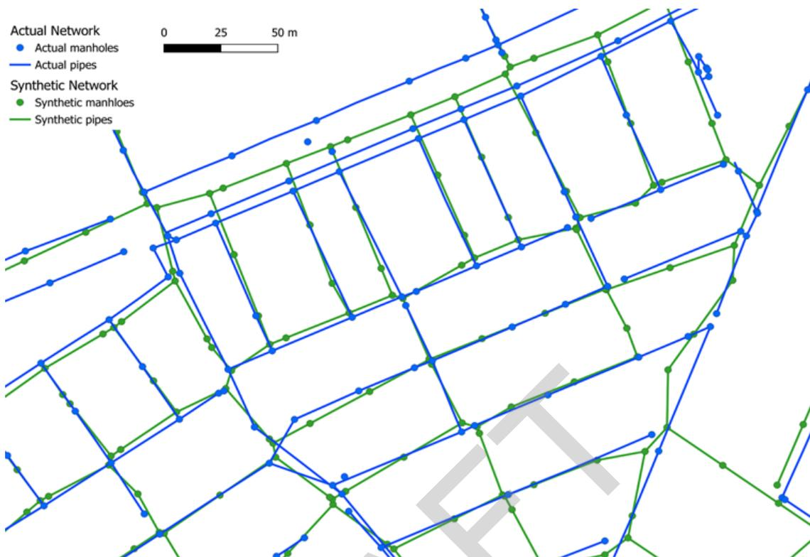
**Figure 10:** Detailed view of the synthetic and the actual network.
