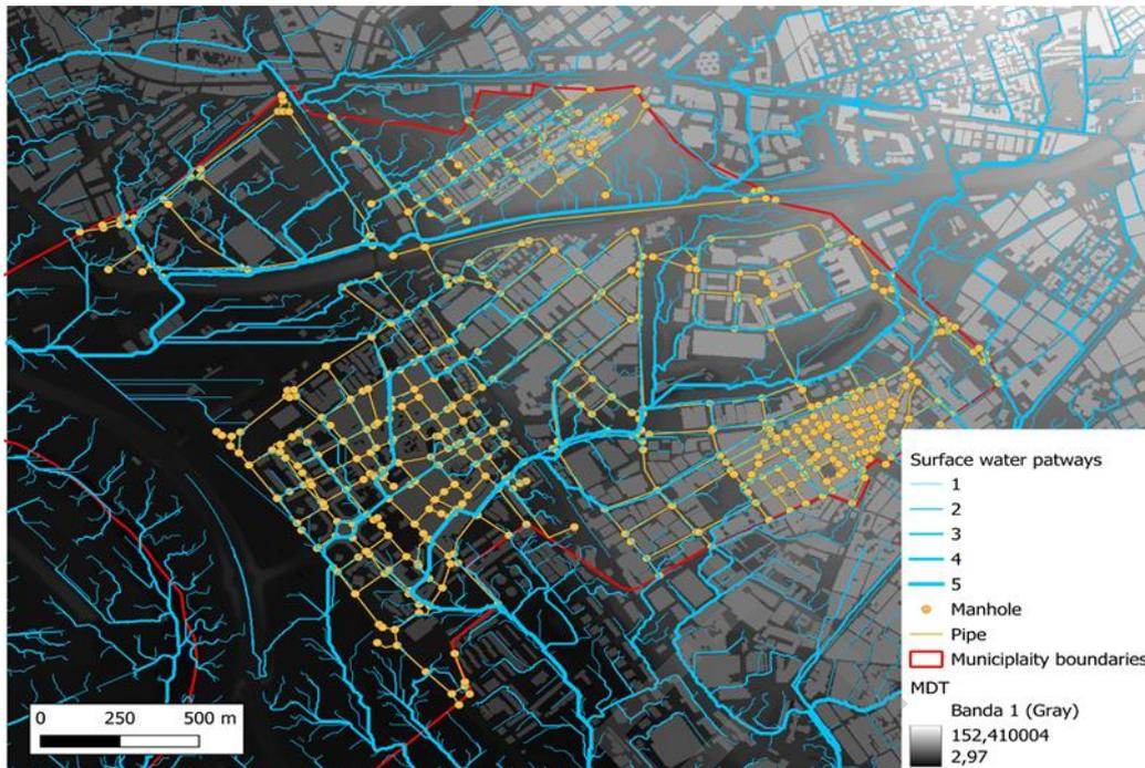
**Figure 12:** Shreve classification of the superficial water courses in Sant Joan Despí together with the synthetic sewer network generated.
