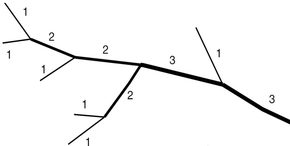
**Figure 11:** Classification of the order of pipes in a basic sewer network following the Shreve classification.
