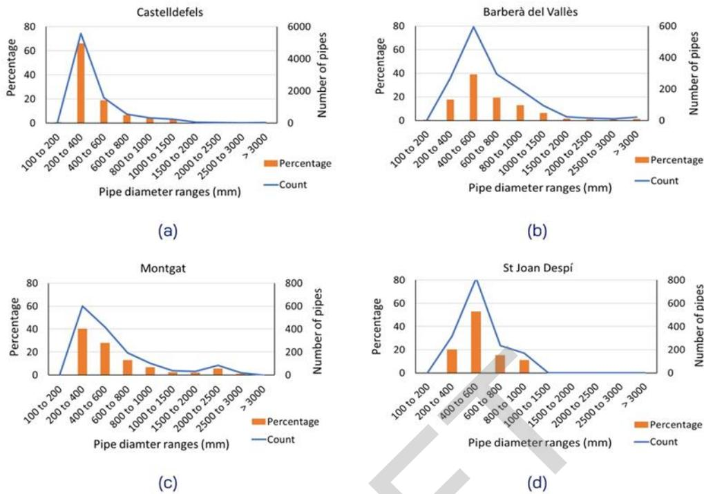
**Figure 8:** Distribution of pipe diameters in the municipal sewer networks of (a) Castelldefels, (b) Barberà del Vallès, (c) Montgat and (d) St Joan Despí.
